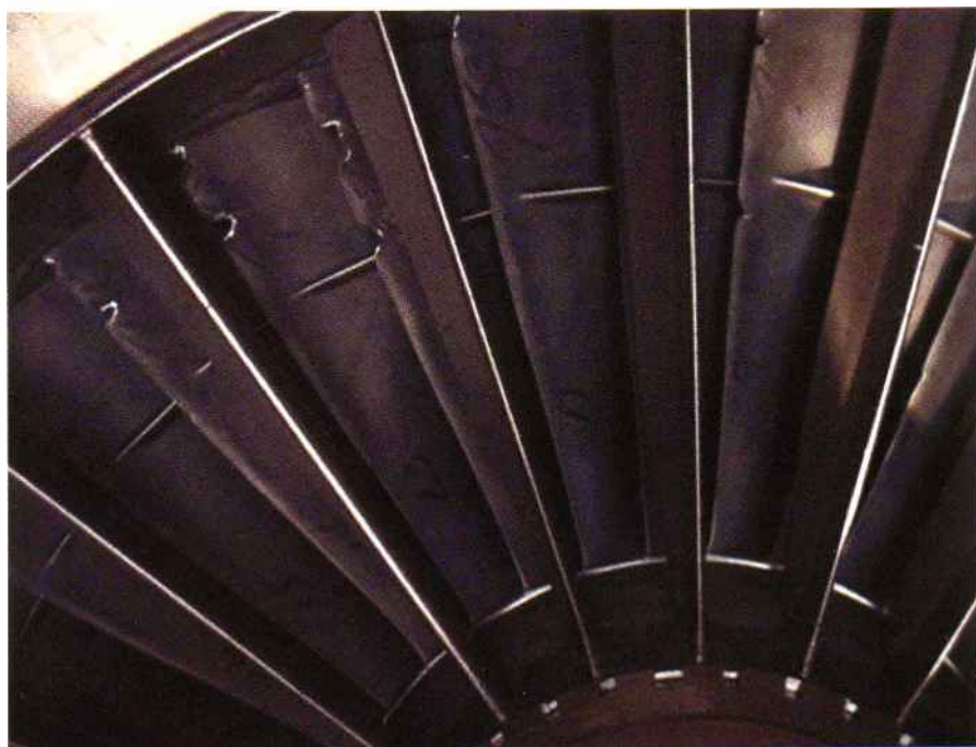
It was estimated from the remains that at least three ducks were ingested into the number one engine causing severe damage to fan blades throughout the engine.
